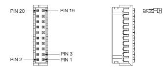
Order kit part number 73-788-002 for control connector interface with unloaded housing and 20 pins
